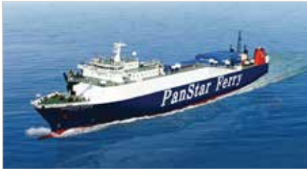
SANSTAR DREAM - Gross Ton : 11,820M/T - L.O.A : 149.57M - Speed : 21.50kn - Cargo Capacity : 210TEU
