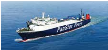
SANSTAR DREAM - Gross Ton : 11,820M/T - L.O.A : 149.57M - Speed : 21.50kn - Cargo Capacity : 210TEU
