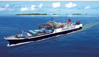
M/V PANSTAR GENIE NO.2 Gross Ton : 13,681M/T L.O.A : 161.15M Speed : 18.00kn Cargo Capacity : 264TEU
