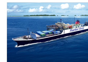
M/V PANSTAR GENIE NO.2 Gross Ton : 13,681T L.O.A : 161.15M Speed : 18.0KN Cargo Capacity : 264TEU
